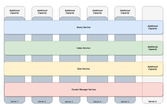
Figure 3.1.2.1 The homogeneous scaling model of Couchbase Server
